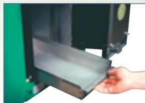
The ash is collected in a ash tray in the bottom of the combustion chamber. Just to pull out and empty.
