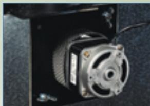
The suction fan is easily accessible from the backside for sweeping and service.
